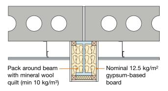
An alternative detail where two steel beams are required to support the external cavity wall is as follows:
