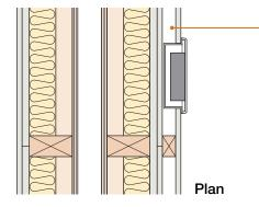
Alternatively provide a service void on surface of separating wall. This is the preferred method where more than one socket, switch, etc. are close together, e.g. in a kitchen.
