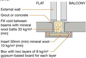
Separating walls should not be constructed off steel beams.
